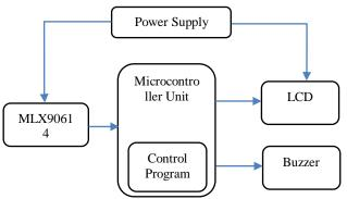
Figure 1: Block diagram of the designed NCFIT
