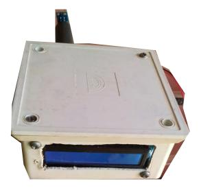
Figure 4: Constructed Non-Contact Forehead Infrared Thermometer
